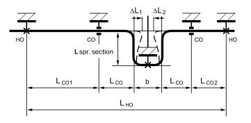
The compensation of thermal extensions is solved constructively, using angles of rotation, sliding and fixed supports, as well as ready-made expansion joints. In fixed supports, the pipe is rigidly fastened with a collar with rubber gasket, and in sliding supports, retainers allow the pipe to move in the axial direction.
