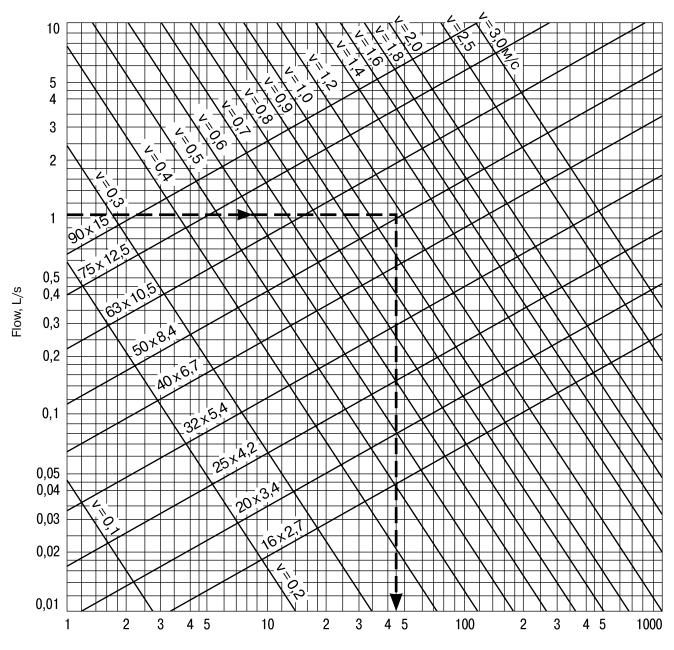
Head loss due to friction, mm/m
