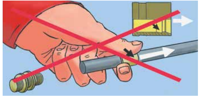
The sleeve is put on "the wrong way": the chamfer inside the sleeve points in the opposite direction to the fitting
